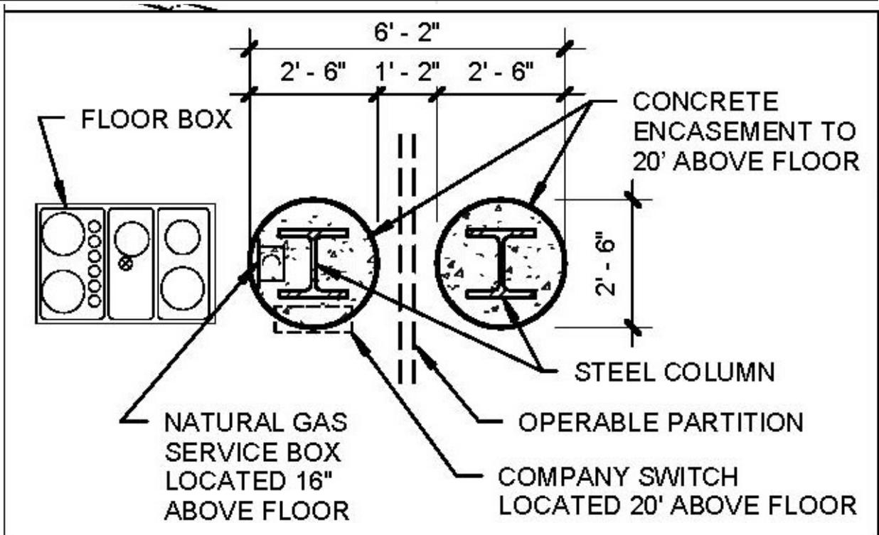
Note: Natural gas service box and Company Switch are always located on column closest to floor box.
